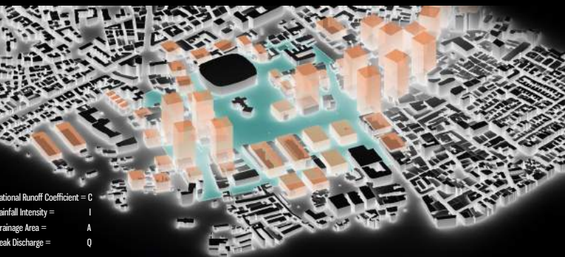
Using the Rational Method for design flood events to calculate runoff water volumes in various scenarios
